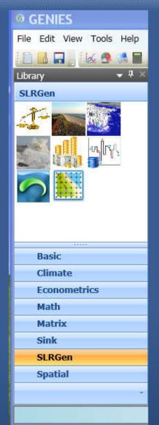
Each block in the library can be dragged into the canvas to be configured and used as a component of a model, the blocks can be linked to each other according to their data and function nature.
